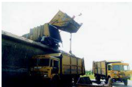
Transfer of waste from Compactor to Bulk Refuse Carrier at Hadapsar Ramp
